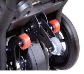
The new rear support is adjustable according to the different heights of steps increasing the security and stability without the need to seek the point of equilibrium.
